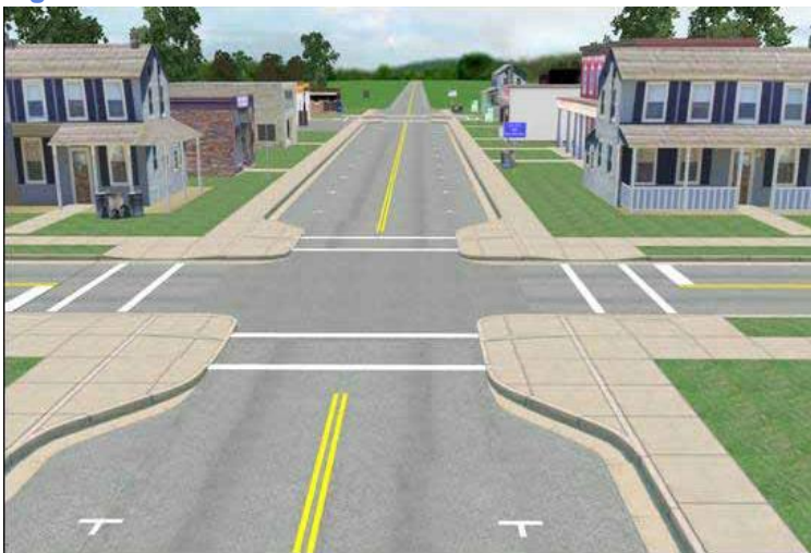
Figure 38: Curb Extension on Side Streets
