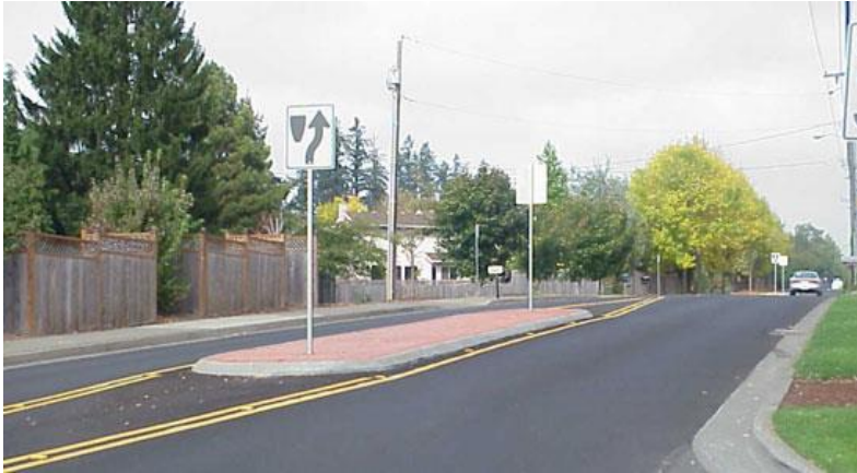
Figure 35: Raised Median Example
